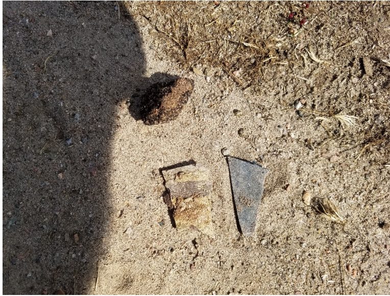
ACM Floor Tile, ACM Mastic on Brick and Non-ACM Step Tread
