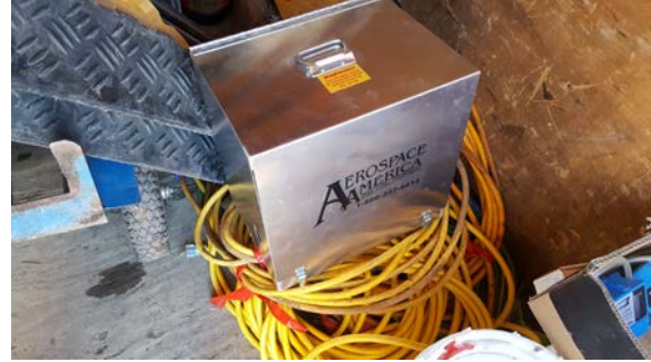
5 micron water filtration system used to filter water used to clean the excavator bucket.
